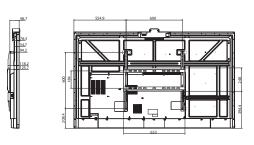
**86"** Product Size (W x H x D): 1954.7 x 1197.6 x 125.9mm / 77 x 47 x 5.0inch Package Size (W x H x D): 2005 x 1202 x 210 **Package Size (W x H x D):** 2095 x 1303 x 240mm / 82.5 x 51.3 x 9.4inch Net Weight: 59.0kg / 130.1lbs Packed Weight: 76.5kg / 168.6lbs
