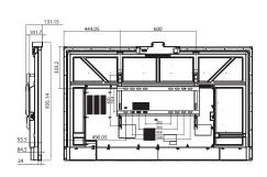
75" Product Size (W x H x D): 1709.9 x 1060.1 x 125.9mm / 67.3 x 41.7 x 5.0inch **Package Size (W x H x D):** 1850 x 1165 x 240mm / 72.8 x 45.9 x 9.4inch **Net Weight:** 45.8kg / 101.0lbs **Packed Weight:** 60.0kg / 132.3lbs
