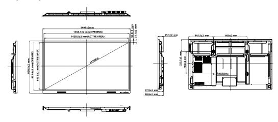
75" Product Size (W x H x D): 1712 x 1022 x 99mm / 67.4 x 40.2 x 3.9inch **Package Size (W x H x D):** 1863 x 1155 x 185mm / 73.3 x 45.5 x 7.3inch Net Weight: 41.8kg / 92.2lbs Packed Weight: 53.4kg / 117.7lbs
