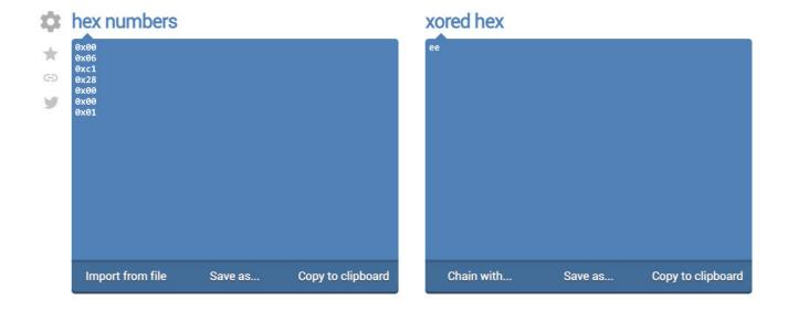
The value of "xx" (the check bit) will change as you alter the ID of the screen you wish to control. So the value of "xx" is not the same for controlling a screen with an ID of 01 and a screen on ID 22 for example. So the code sent to the screen for control is different.
