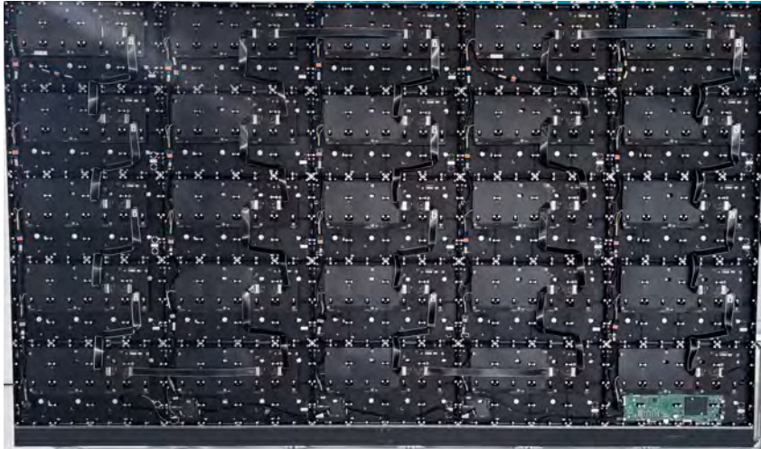
FFC signal cables connection for HAIO136GE(five by five)
